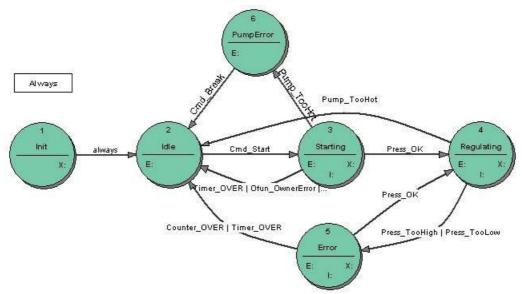
Figure 2 StateWORKS: Representation of a state transition diagram
