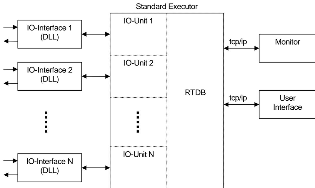
The heart of the system is the Standard Executor which contains the RTDB and IO-Units. Each IO-Unit is the same. The number of IO-Unit incarnations is defined by specifying the control system in the StateWORKS Studio. Though the code of IO-Units is the same the number of inputs and outputs may differ and is configured by system specification.
