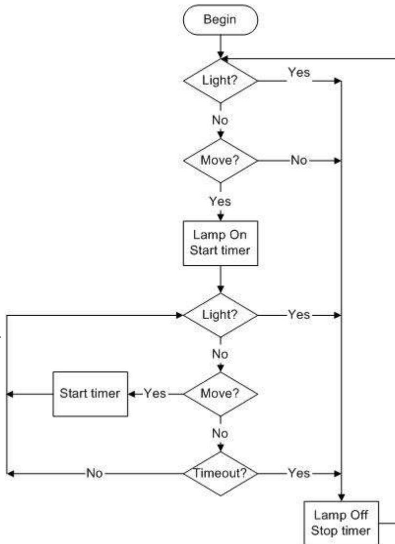
Figure 5 Flowchart of the Security lamp control
