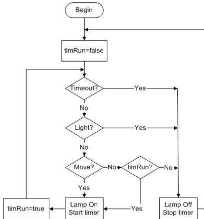
Figure 6 Flowchart of the Security lamp control: solution with a flag
