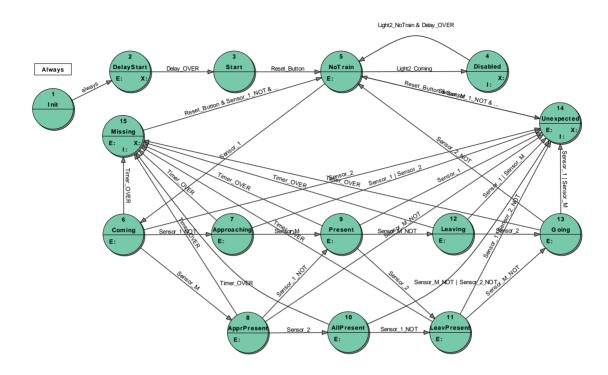
The state transition diagram displays only the states and transition conditions. The complete specification requires the entry, exit and input actions which are only indicated the diagram by letters E:, X;, I;. The full specification is included in state transition tables. (If you explore the design by means of StateWORKS Studio, you will need to double-click on any state to see the full details of its actions and transitions.)
